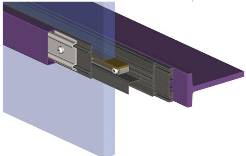
The main grid profiles are produced from a hot rolling process using high-quality ST37-2 grade steel. The system is available with 50mm or 60mm wide sight lines with differing web thickness' and depth dimensions to suit the application.
