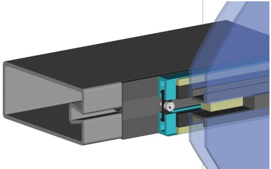
The SG blast resistant curtain walling system offers a significant development in the design of blast mitigation glazing systems. Utilising grid profiles from the 60mm wide SR curtain walling range, the system is designed as a semi unitised, structurally glazed system.
