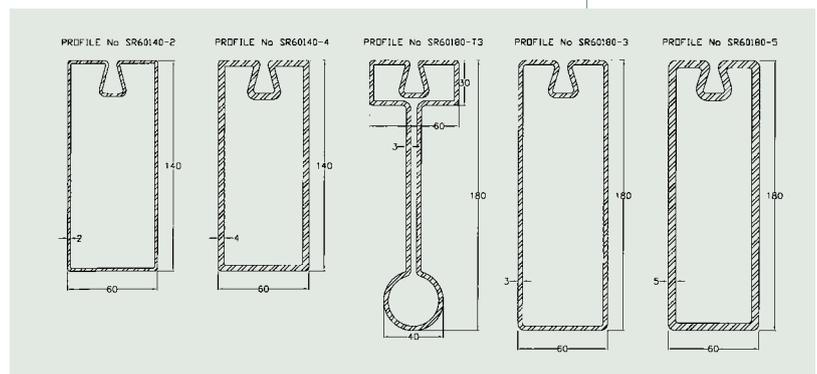
The narrow 60mm sightlines, in combination with the structurally glazed exterior gives the appearance of any other non-specialised glazed assembly, enabling the designer to move away from the traditional wide profiles normally associated with blast resistant applications.
