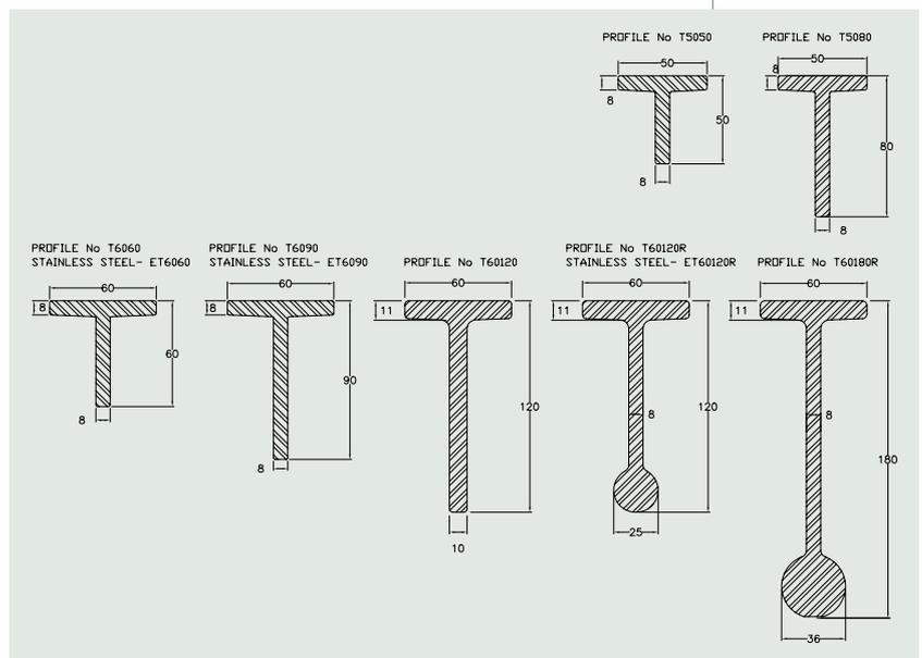
Benefiting from the solid form of the profile, extremely large expanses of glazing can be achieved due to the high static values of the steel.
