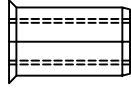
PART No H10099 M6 INSERT C/S FOR 2MM TO 4MM WALL THICKNESS
