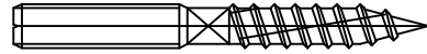
PART No WZ0112 STAINLESS STEEL M6 50MM SCREW (PART No WZ0113 60MM)
